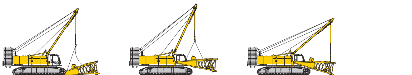
Unloading and assembly of boom foot
